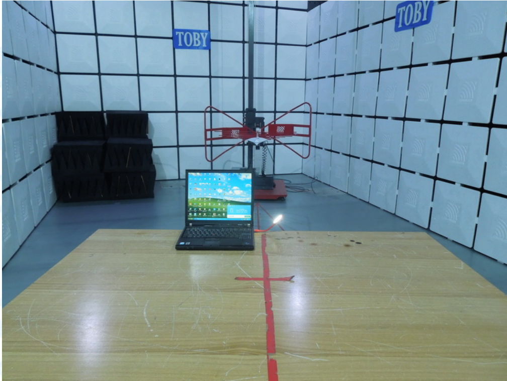
Photo 1 Radiated Emission Test Setup
