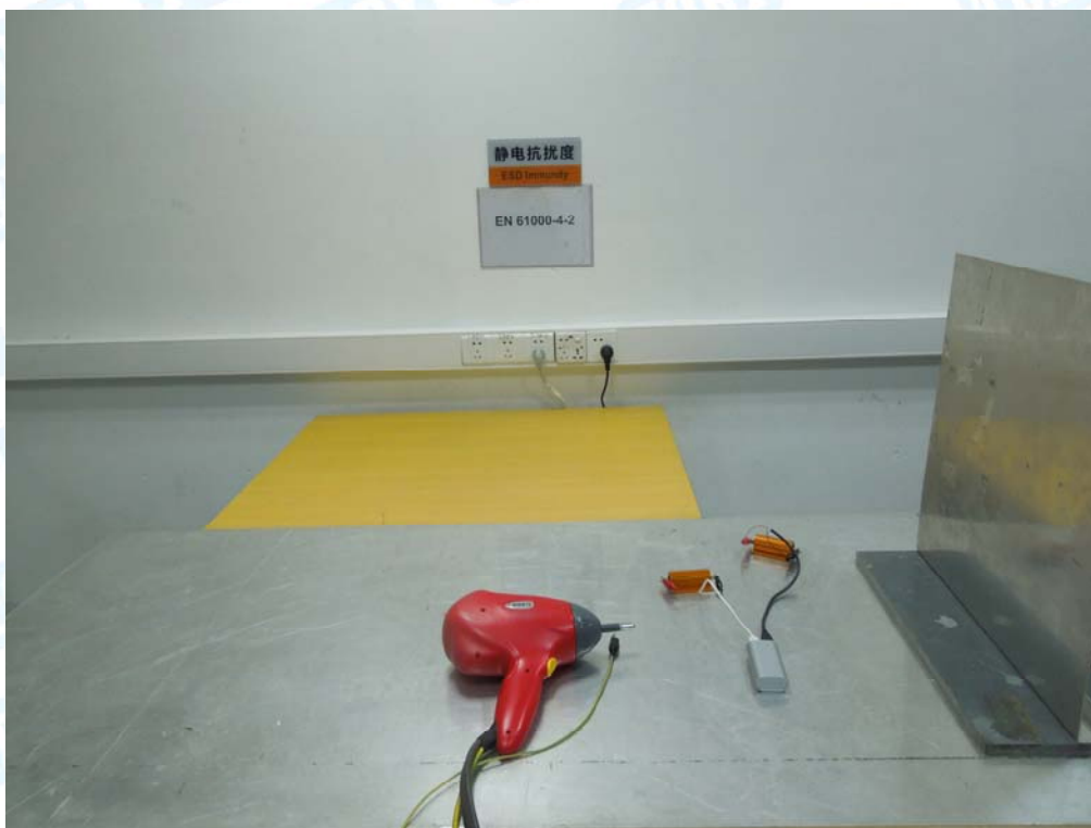
Photo 4 Electrostatic Discharge Test Setup
