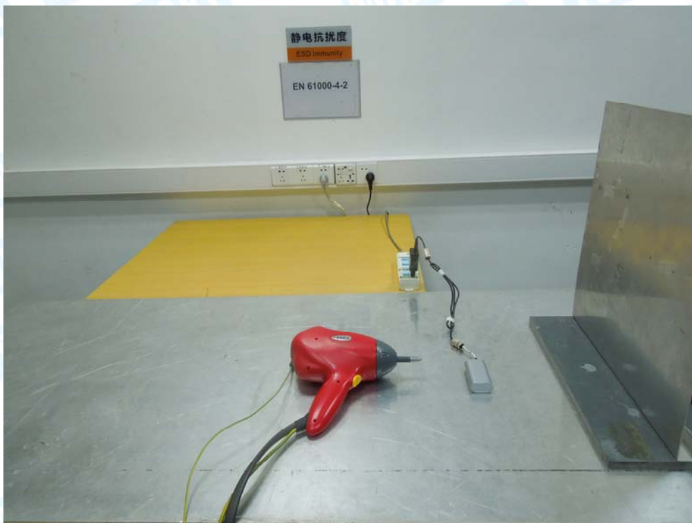
Photo 4 Electrostatic Discharge Test Setup
