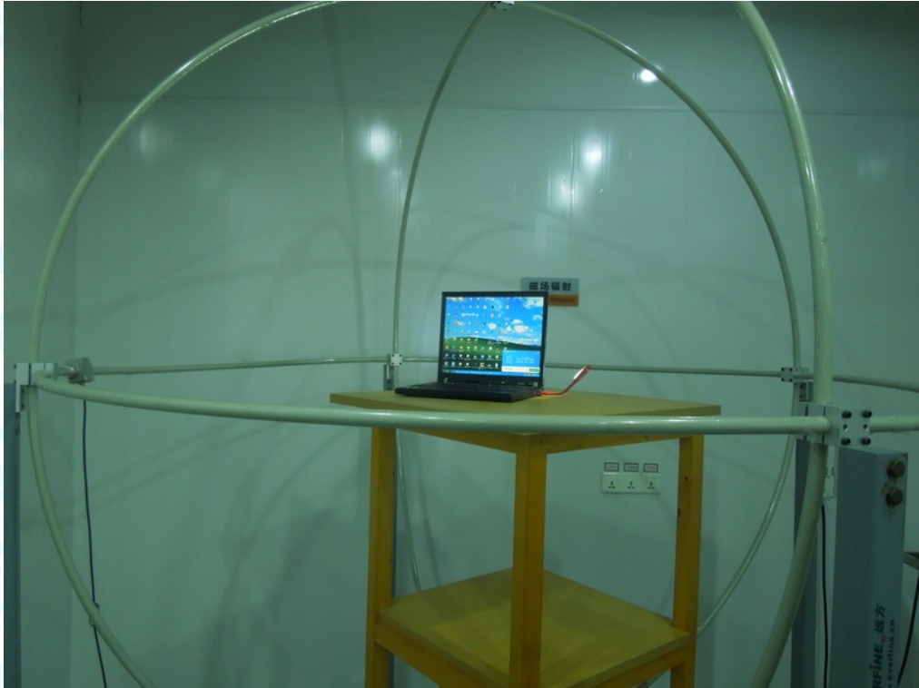
Photo 2 Radiated Emission Test Setup
