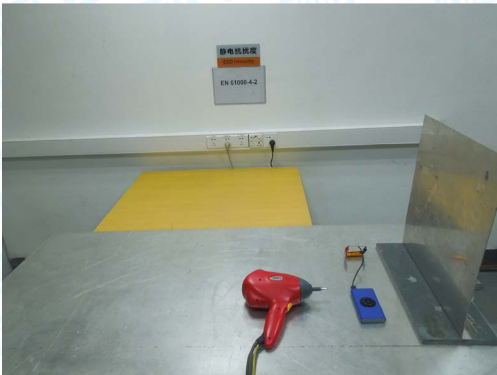
Photo 4 Electrostatic Discharge Test Setup
