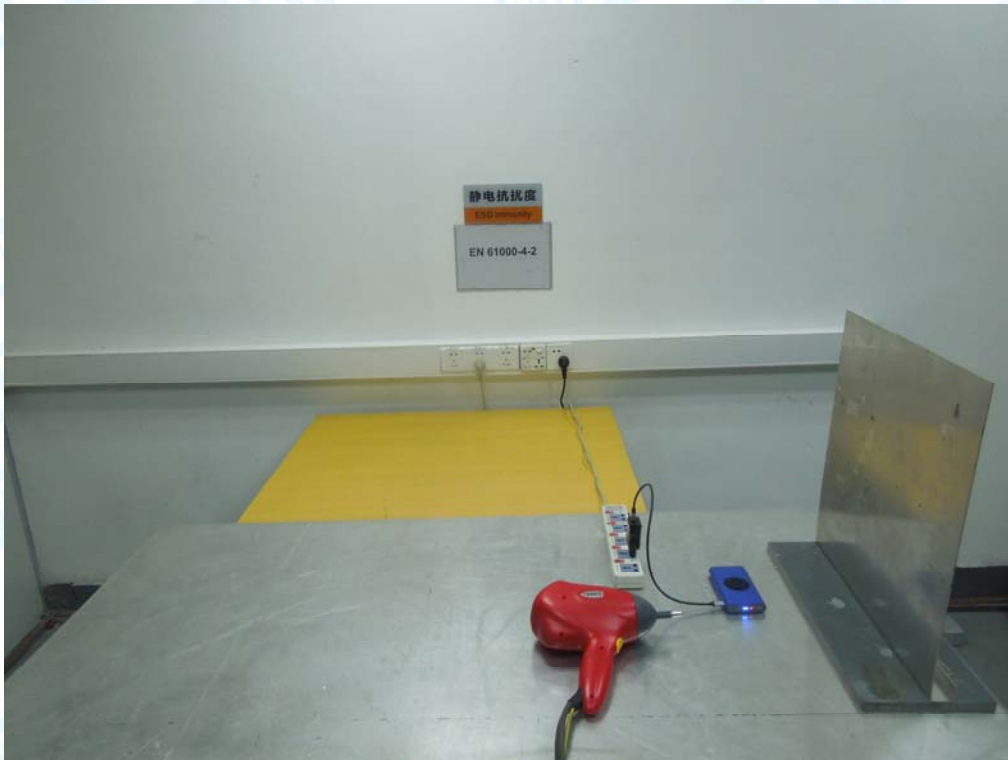
Photo 4 Electrostatic Discharge Test Setup
