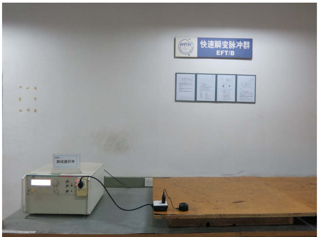
14.6 Photo of Electrical Fast Transient /Burst Test
